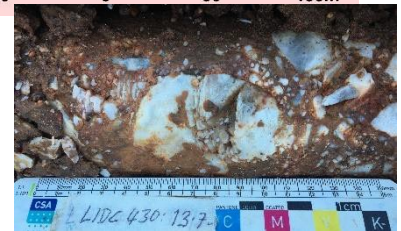
Fault brecciated quartz vein (mod-high Au grade).
