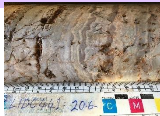
Banded chalcedonic quartz vein (mod-high Au grade).
