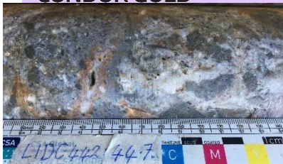
Multi-stage quartz veining (high Au grade).
