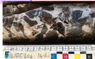
Footwall quartz breccia (low-moderate Au grade).
